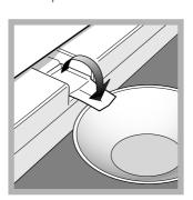
5. Certain appliances are fitted with the DRAIN SYSTEM to lead the water outside. Let the water flow into a container (see diagram).
